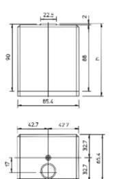
h: The dimensions differ according to the type of socket: 95 with socket A 99 with socket B 98.3 with socket N
