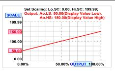
The range between **Ao.HS** and **Ao.LS** should be over 20% of span at least; otherwise, it will be got less resolution of analogue output.
