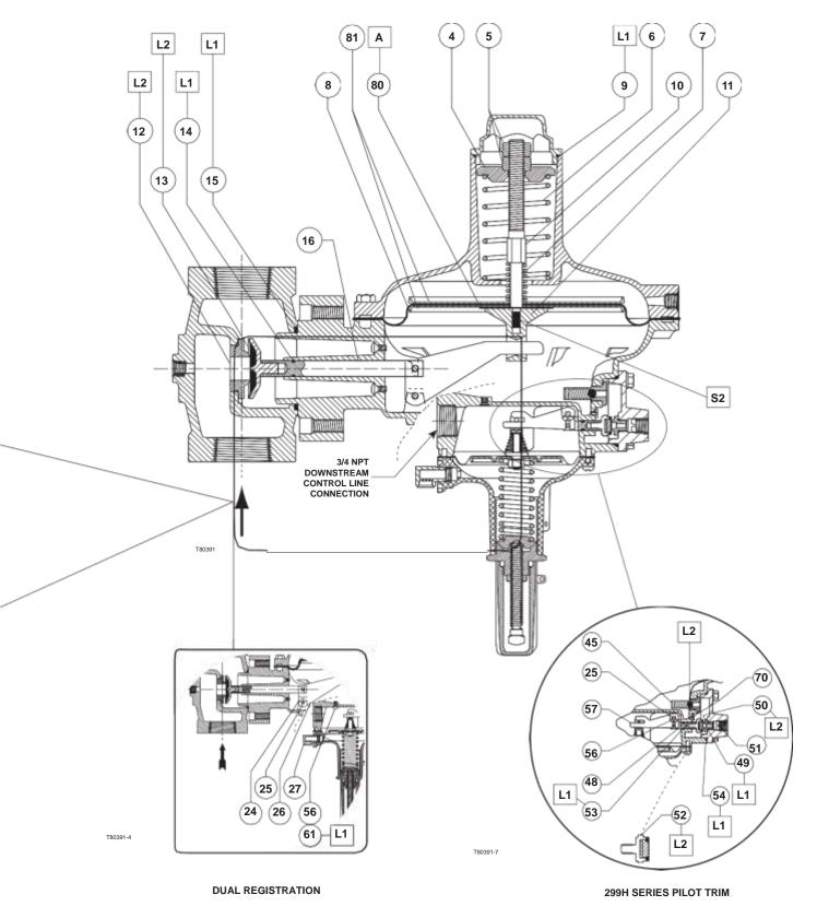
☐ APPLY MULTI-PURPOSE LUBRICANT (L1) / ANTI-SEIZE COMPOUND (L2) / THREAD LOCK SEALANT (S1) / ADHESIVE (A)
