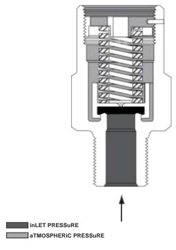
Figure 2. H100 Series Operational Schematic
