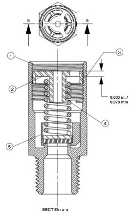
Figure 3. H100 Series Assembly Drawing
