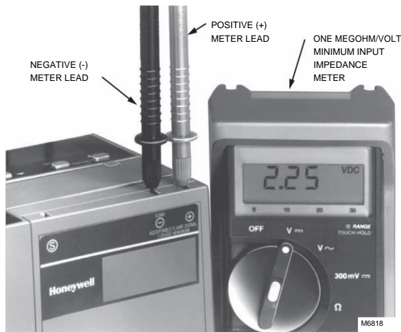
Fig. 11. Measuring voltage flame signal with 7800 SERIES controls.
