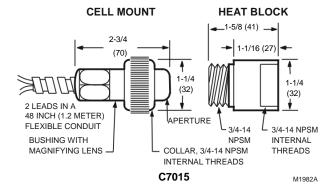
Fig. 3. Infrared detector dimensions in in. (mm).
