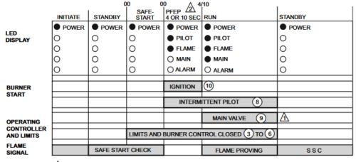
MAIN FUEL VALVE WILL BE ENERGIZED DURING PFEP IF FLAME IS PROVEN.
