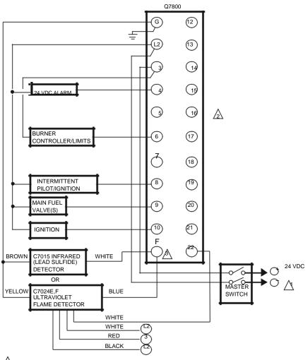
124 VDC POWER SUPPLY. PROVIDE DISCONNECT MEANS AND OVERLOAD PROTECTION AS REQUIRED.
