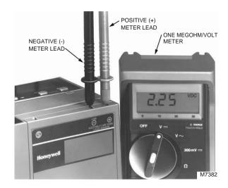
Fig. 17. Flame signal measurement.
