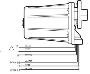
FLAME DETECTOR LEADS ARE COLOR CODED. THE BLUE LEAD MUST BE CONNECTED TO THE F TERMINAL AND THE YELLOW MUST BE CONNECTED TO THE G TERMINAL. THE UV SENSING TUBE IS POLARITY SENSITIVE. REVERSING THE LEADS EVEN MOMENTARILY CAN DAMAGE OR DESTROY THE UV TUBE.
