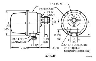
Fig. 4. Rectification detectors in in. (mm).
