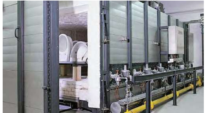
Ceramics industry: intermittent shuttle kiln
