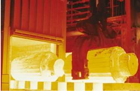
Metallurgical industry: forging furnace
