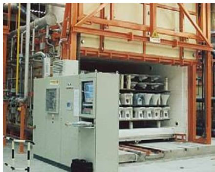
Intermittent shuttle kiln in the ceramics industry
