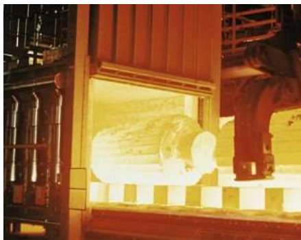
Bogie hearth forging furnace in the metallurgical industry
