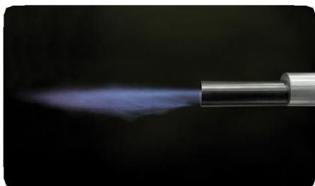
Flame of the ZKIH during natural gas operation in the open air
