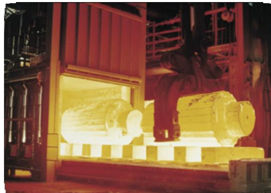
Bogie hearth forging furnace
