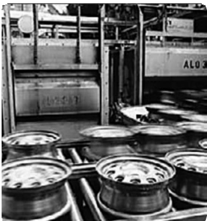
Wheel rim hardening installation
