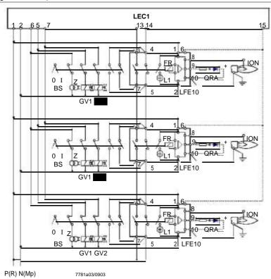
Like with dual-supervision, the control contacts of the flame relays of all flame safeguards must be connected in series when using multiflame supervision.
