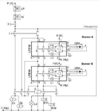
With this type of supervision, too, the burner can be started only if the flame detector or flame simulation test has been successful. This means that **neither** of the 2 flame safeguards may detect a flame signal during burner off times. When the burner is started up, the detector test will automatically be interrupted.
