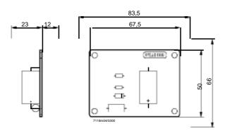
Remote lockout reset module for use with the LOA26... / LOA36...
