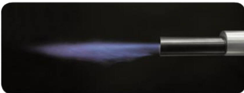
Flame of the ZKIH during natural gas operation in the open air
