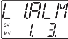
Alarm 1 and 3 are activated
