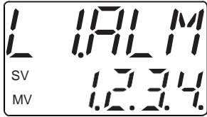
Alarms 1 to 4 are all activated
