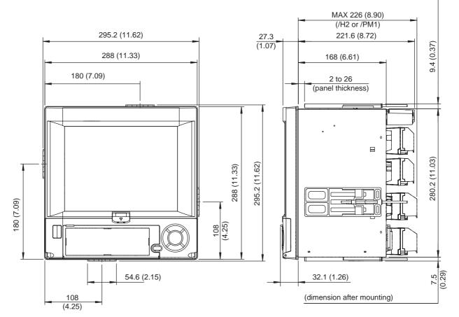
Note: If not specified, the tolerance is  $\pm$ 3%. However, for dimentions less than 10mm, the tolerance is  $\pm$ 0.3mm.
