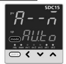
Press and hold [para] for more than 2s to get the parameter setup display.
