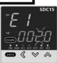
When [<],  $[\lor]$  or [^] is pressed, the rightmost digit on the lower display flashes, and can be changed to the desired value for the event. In this case, the flashing of the numerical value implies that it is not yet set. A numerical setting that is being changed flashes the same way.
