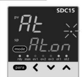
If no key is pressed for more than 2s, remains steadily lit and AT begins. During AT, the rightmost decimal point flashes twice repeatedly. (When AT is done, the light goes off and the new PID values go into effect.)
