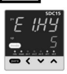
To set hysteresis as well, press [v] twice or press [] repeatedly to get £ 1.35 on the upper display and 5 on the lower display.
