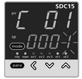
When the [<],  $[\lor]$ or [\Lambda] key is pressed, the rightmost digit on the lower display flashes. If no key is pressed for more than 2s after changing to the desired value in the PV input range list, the display changes from flashing to continuously lit, and the displayed value is now set.
