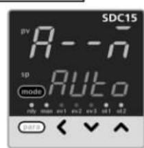
Press and hold [para] for more than 2s to get the parameter setup display.
