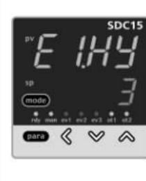
When [<], [v] or [\lambda] is pressed, the rightmost digit on the lower display flashes, and can be changed to the desired value for hysteresis.
