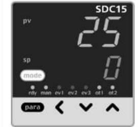
Start from the operation display (if necessary press [mode] once to get the operation display).
