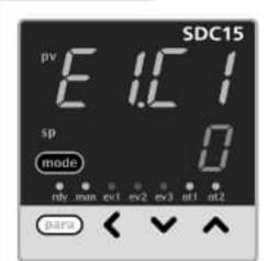
Press [para] repeatedly to get £ 1.5 f on the upper display. 5 is displayed on the lower display.
