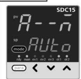
Press and hold [para] for more than 2s to get the parameter setup display.
