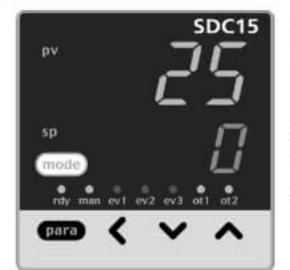
Start from the operation display (if necessary press [mode] once to get the operation display).
