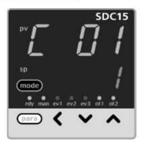
Press and hold [para] for more than 2s again to get the setup setting display. The current set value for [] (PV input range type) is displayed.
