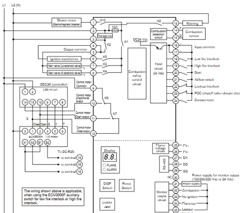
Note: - Use contact reset (terminal 24) input in isolation. It cannot be used in conjunction with other BC-R contact reset inputs.
