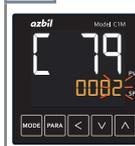
Press [**<**], [**V**], or [**^**]. The lower display flashes. Change to the desired setting by pressing [**V**] or [**^**]. Do not press any key for 2 s. The new value stops flashing and is now set.
