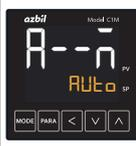
Press [MODE] once to show the operation display, and then hold down [PARA] for 2 s or longer.
