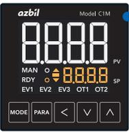
Power-on → all on → all off → sequential on and off → operation display (sequence takes about 9 s)
