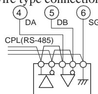
Example: Method to connect with a 5-wire type instrument
