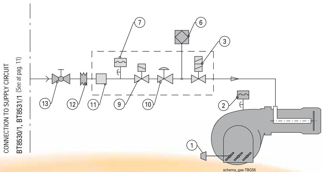
**DIAGRAM FOR THE CONNECTION OF A BURNER TO THE GAS MAINS AT AVERAGE PRESSURE (BT 8531/1)**
