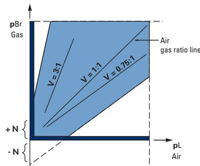
N = Regulates air-gas ratio at minimum capacity (origin of ratio line).
