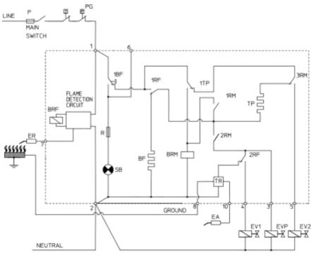
**BRM** Operation relay EV1 First main valve **BRF** Flame detection relay EV2 Second main valve BF Safety time thermal **EVP** Pilot valve EΑ Ignition electrode SB Lockout signal ER Detection electrode TP Waiting time thermal
