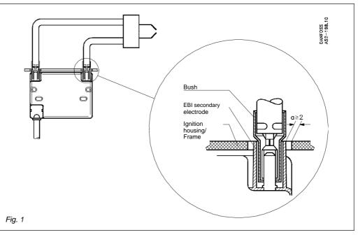
The insulation property of ignition cables depends on the material used and the thickness of the insulation. If cables with insufficent insulation are used, especially together with divergent electrodes, there is a risk of electrical insulation breakdown should the cables
