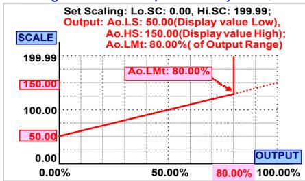
**Fine zero & span adjustment:**
