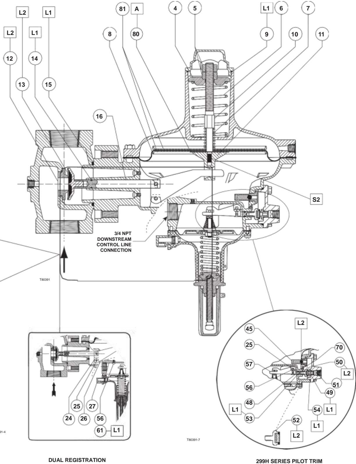
□ APPLY MULTI-PURPOSE LUBRICANT (L1) / ANTI-SEIZE COMPOUND (L2) / THREAD LOCK SEALANT (S1) / ADHESIVE (A)
