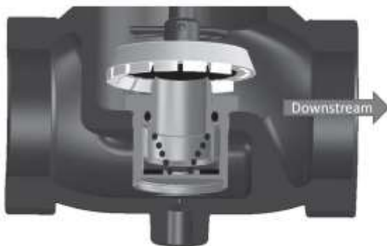
Figure 7. White Disk Orientation for use with Secondary Seat™ Protection
