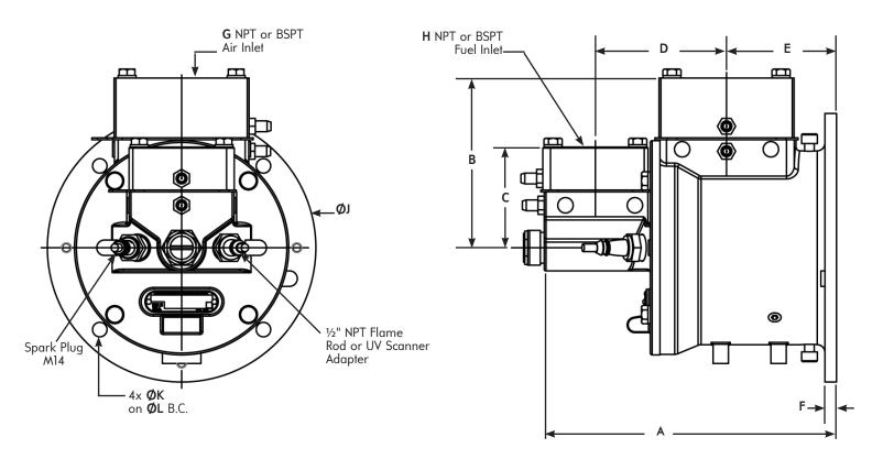
5A/5B Burner weight less tile: 28 lbs. (12.7 Kg) 6A/6B Burner weight less tile: 39 lbs. (17.7 Kg)
