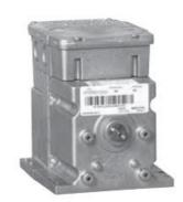
The Series 72 Modutrol IV Motors spring return and non-spring return motors are used to control dampers and valves. The motors accept a current or voltage signal from an electronic controller to position a damper or valve at any point between open and closed.
