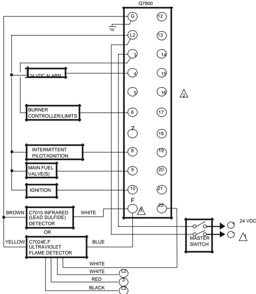
⚠ 24 VDC POWER SUPPLY. PROVIDE DISCONNECT MEANS AND OVERLOAD PROTECTION AS REQUIRED.
