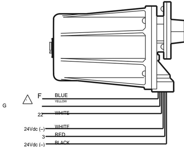
⚠️ FLAME DETECTOR LEADS ARE COLOR CODED. THE BLUE LEAD MUST BE CONNECTED TO THE F TERMINAL AND THE YELLOW MUST BE CONNECTED TO THE G TERMINAL. THE UV SENSING TUBE IS POLARITY SENSITIVE. REVERSING THE LEADS EVEN MOMENTARILY CAN DAMAGE OR DESTROY THE UV TUBE.
