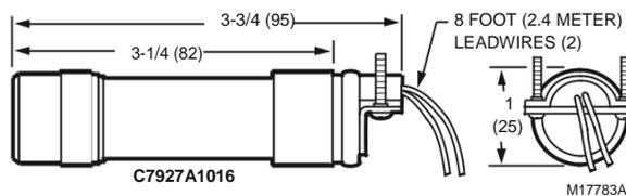
**Fig. 5. C7927 detector dimensions in in. (mm).**
