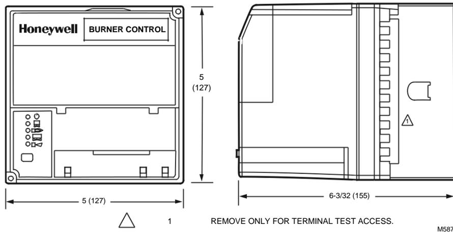
Fig. 2. Mounting dimensions of RM7824A Relay Module and Q7800B Subbase in in. (mm).
