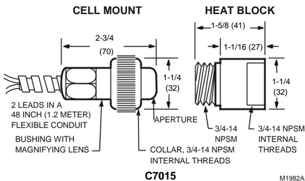
Fig. 3. Infrared detector dimensions in in. (mm).
