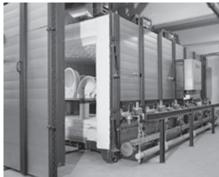
Intermittent shuttle kiln in the ceramics industry
