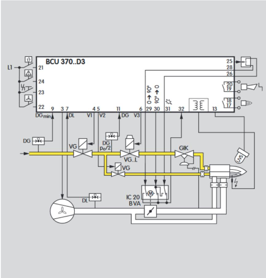
**Modulating-controlled forced draught burner with pilot burner and tightness control**
