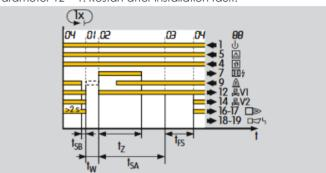
If the BCU detects an installation fault (flame failure or failure of air flow) after a minimum operating time of 2 s.
