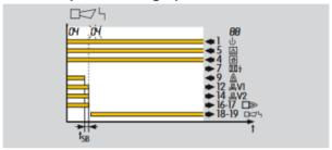
If the flame fails during operation, the valve outputs are disconnected within the safety time tsp.
