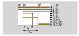
If no flame forms or, in the case of BCU 465, if the air flow fails during start-up, a fault lock-out is performed after expiry of time  $t_{\text{SA}}$ . The display blinks and shows the cause of the fault.
