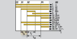
After the start-up signal (3) has been applied and after the flame simulation check and "no flow" state check have been conducted successfully, the air valve is opened. Start-up of the burner commences as usual with no interruption of the air after expiry of the
