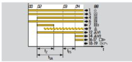
If the temperature in the furnace chamber drops below 750°C, the DI input must be disconnected from the electrical power supply and the furnace must then be operated with flame control.
