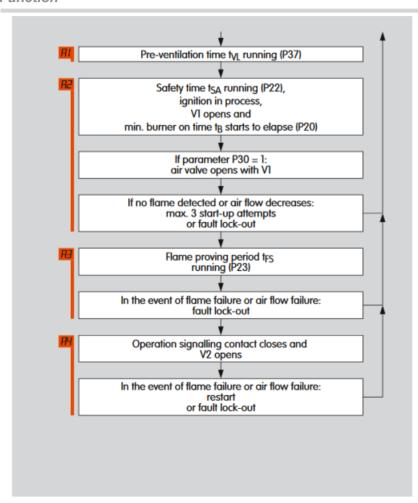
If both flame and air flow are detected during the safety time t<sub>SA</sub>, the flame proving period t<sub>FS</sub> starts after this safety time has elapsed. Valve V2 opens and the operation signalling contact between terminals 16 and 17 closes. This completes start-up. An adjustable min. burner on time t<sub>B</sub> ensures that the burner burns for a defined period even if the start-up signal (3) is switched off beforehand.
