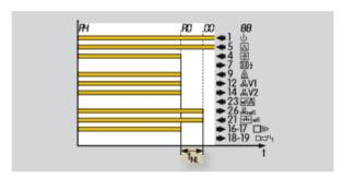
The air valve remains open for the programmed time after the start-up signal ( $\vartheta$ ) has been deactivated. The burner control unit closes the air valve after expiry of the post-ventilation time tNL.
