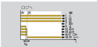
After an installation fault (flame failure or failure of air flow), the burner control unit performs a fault lockout within the safety time during operation tsB. This involves disconnecting the power from the gas valves and, if applicable, the ignition transformer. The fault signalling contact closes, the display blinks and shows the current program status, see table on page 39 (Program status and fault messages).
