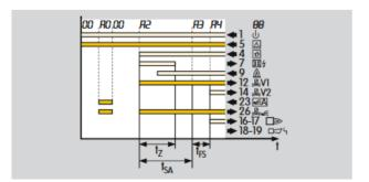
Parameter 30 = 1: The air valve opens simultaneously with valve V1.
