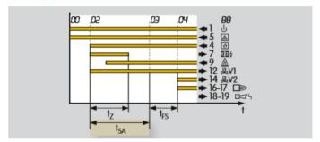
This indicates the safety time on start-up  $t_{\text{SA}}$  for the burner.
