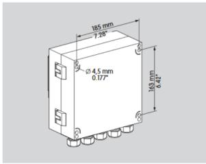
Die-cast aluminium housing with plug-in terminal blocks and plug-in M20 cable glands or (16-pin) plug connector for input signals and optionally pre-assembled cables for output signals.
