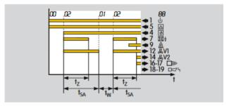
If several start-up attempts are set at the works and if the BCU detects an installation fault during start-up, it closes valve V1 after the safety time  $t_{SA}$  has expired and
