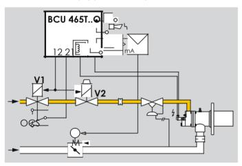
Parameter 09 = 1: A signal is sent to the BCU via the position indicator on the gas solenoid valve V1 stating whether the valve is closed or open. In standby, the switch must be closed. During start-up and operation, the switch must be open. This ensures that valve V1 is open or closed.
