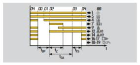
An immediate restart of the burner after a controlled shut-down is prevented by the pause time. The pause time starts when the burner is switched off. If a start-up signal (3) is applied before expiry of this time, start-up is delayed until the end of the pause time.
