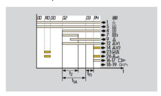
Parameter 30 = 2: The air valve opens simultaneously with valve V2.
