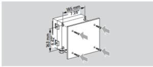
Screw on the closed unit to the rear with 4 self-tapping screws (enclosed).
