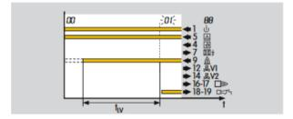
An extraneous signal (flame simulation) is a flame signal that is detected, although there should be no flame according to the program sequence. If such an extrane-ous signal is detected, the flame simulation delay time tLV starts to elapse. If the flame simulation is discontin-ued during the flame simulation delay time tLV, start-up can be initiated or operation continued. Otherwise, a fault lock-out occurs.
