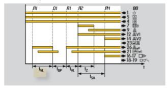
With this function, the combustion chamber can be purged after a safety shut-down in compliance with standards, especially on radiant tube burners. This task is not implemented by a central control system but by the BCU 465. See also parameters 40 and 41.
