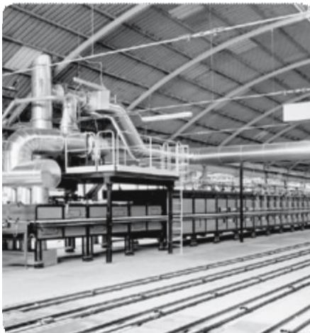
Roller hearth kiln in the ceramics industry
