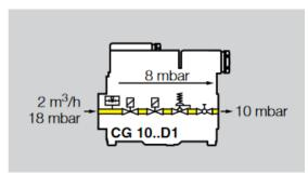
The operating point P1 (V'max. = 2 m3/h;  $\Delta p$ = 8 mbar) must lie in the working range of the combination control CG 10.
