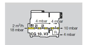
A further 4 mbar must be generated by flow rate adjustment, in addition to the computed pressure drop  $\Delta p = 4$  mbar, in order to achieve the required outlet pressure pG = 10 mbar.
