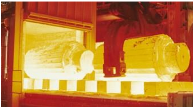
Metallurgical industry: forging furnace
