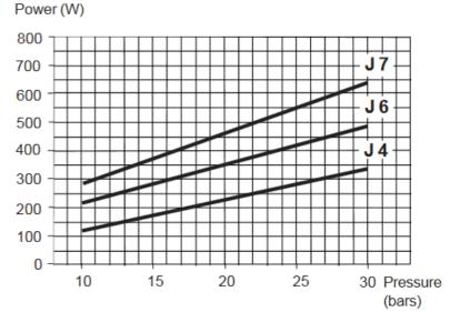
Viscosity = 5 cSt - Rated speed = 2850 rpm
