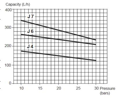
Viscosity = 5 cSt - rated speed = 2850 rpm
