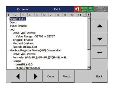
**Custom Edited Display:** In Plus versions, PC software Panel Studio allows users to edit the specific display instead of standard one, and then download it onto PR recorders.
