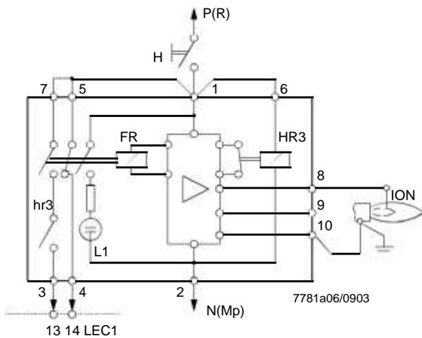
**LAE10 with silicon photocell detector RAR9...**
